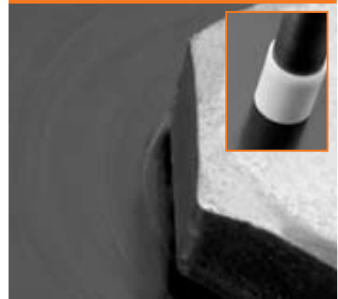
Static covered socket – Light Damage
